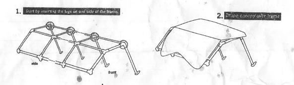
Insert the remaining legs and finish attaching cover to frame.
